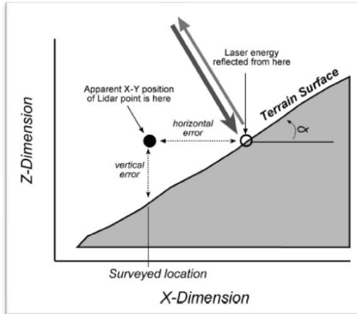
**Figure 5: Illustration of the effects of terrain slope on observable elevation error.**
