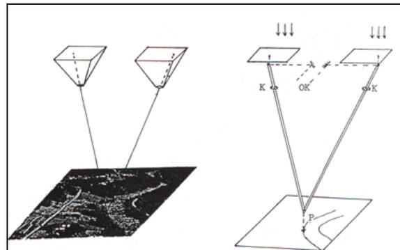
**Figure 4: Concept behind the use of a pair of stereo images for stereo-plotting or image interpretation**
