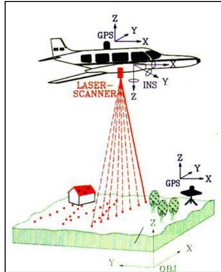
**Figure 2: LiDAR data collection process**
