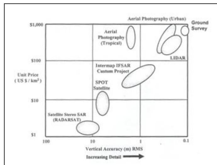
Figure 1: Unit cost comparison of DTMs as a function of typical vertical accuracies addressed by various technologies Source: El-Sheimy *et al.* (2005).
