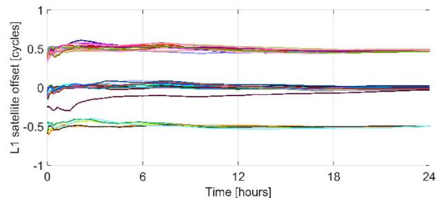
**Figure 6: Convergence of the DCM L1 satellite offsets with respect to the IRC for DOY 179, 2016 with the differences in axis convention not account for. Each colour represents a different satellite with the integer component removed from each time series.**
