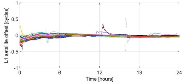
**Figure 5: Convergence of the forward run of DCM L1 satellite offset with respect to the IRC on DOY 178, 2016 with the differences in yaw manoeuvres and axis convention taken into consideration. Each colour represents a different satellite with the integer component removed from each time series.**
