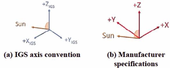
**Figure 2: Orientation of the spacecraft body frame for GPS Block IIR/IIR-M satellites. Sub-plot (a) refers to the manufacturer specification system while sub-plot (b) refers to the IGS axis conventions (Montenbruck et al. 2015).**
