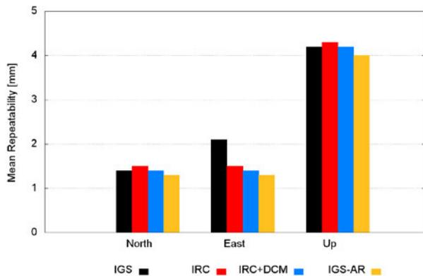
**Figure 15: Examination of the repeatability of the PPP user solution in static mode utilizing different types of clock products. Statistics are based on GPS data from 29 IGS stations were observed during DOY 178 to 184, of 2016. All units are in millimetres.**
