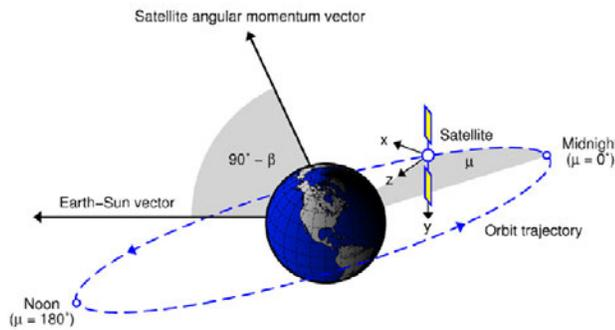
**Figure 3: Geometry of an eclipsing satellite, where  $\beta$  is elevation of the Sun above the orbital plane and  $\mu$  is the spacecraft's geocentric orbit angle. "Midnight" denotes the farthest point of the orbit from the Sun whereas "noon" denotes the closest point. From author Dilssner et al. (2011).**
