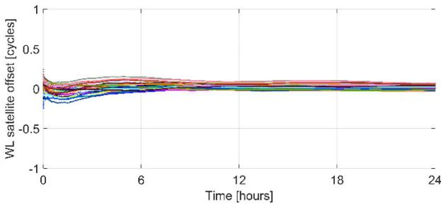
**Figure 8: Convergence of the DCM widelane satellite offset with respect to the IRC on DOY 178, 2016. Each colour represents a different satellite with the integer component removed from each time series.**
