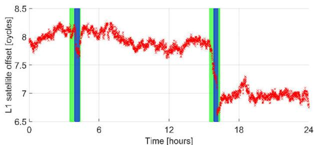
**Figure 4: Inconsistent error modeling during a satellite eclipse for PRN 24, Block IIF on DOY 178 of 2016 between IRC and DCM. The red time series illustrates the unconstrained AC specific satellite offset with respect to PRN 1, the green box illustrates the shadow period provided by JPL and the blue box illustrates the critical yaw manoeuvre provided by NRCan.**
