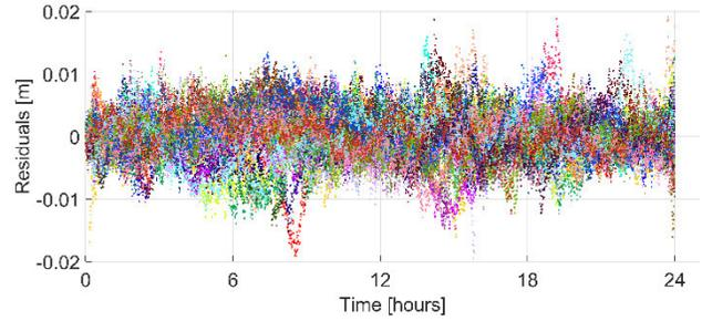
**Figure 10: Post-fit residuals of the combined clock (IRC and DCM) with respect to the reference clock (IRC) on DOY 178, 2016.**
