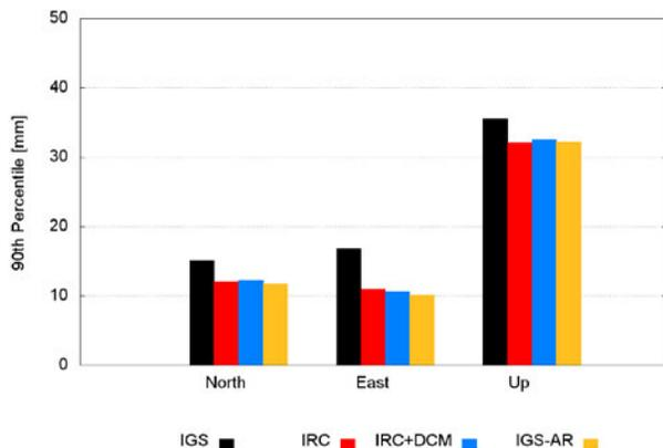
**Figure 16: Examination of the repeatability of the PPP user solution in kinematic mode utilizing different types of clock products. Statistics are based on GPS data from 29 IGS stations were observed during DOY 178 to 184, of 2016. All units are in millimetres.**
