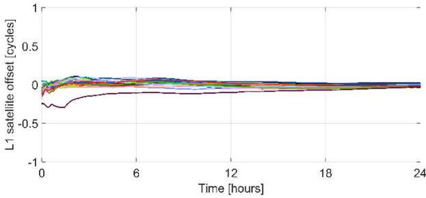
**Figure 7: Convergence of the DCM L1 satellite offset with respect to the IRC on DOY 179, 2016 with the differences in axis convention account for. Each colour represents a different satellite with the integer component removed from each time series.**
