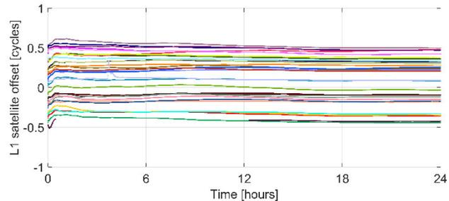
**Figure 11: Convergence of the forward run of IGS L1 satellite offset with respect to the IRC on DOY 178, 2016. Each colour represents a different satellite with an integer component removed from each time series.**
